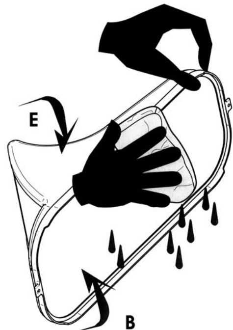
2.4. Wash the inferior part of the base (B), wash the external part (E).
